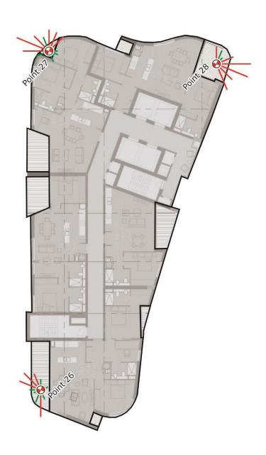
Figure 6d: Wind Directionality Plots – Level 25 – 38 (results shown without any treatments applied)
